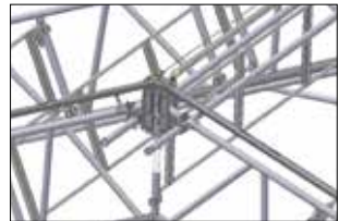
The fall protection anchor in place
