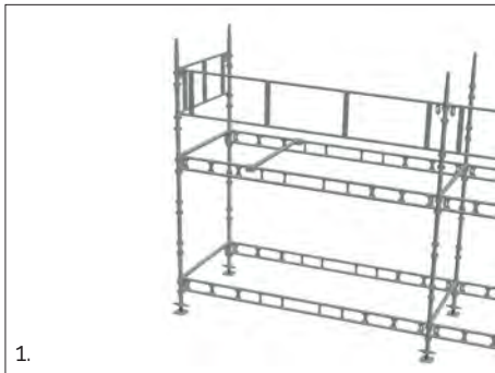
1. Install intermediate transom to support board. More information on page 15 in this manual.
