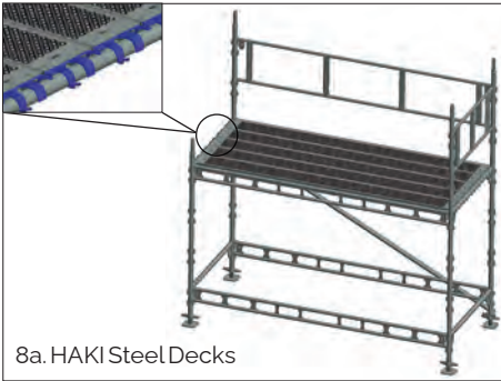
8a. Install HAKI steel decks over the transoms. Prevent uplift by closing locking catch.
