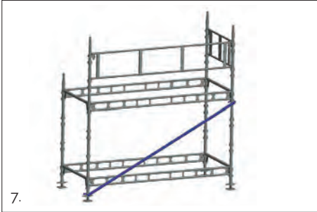
7. Fit facade bracing as requested by the design drawing or as described on page 32 in this manual.
